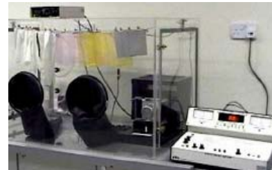
Static Decay Test in Humidity Chamber for Testing under Controlled Environmental Conditions.
