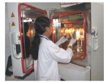
**Thermal Shock** is a mode of environment testing whereby the objects are exposed to a sudde n change in temperature within se conds for a period of time and cycles. Cause by the effect of global warming, the atmosphere temperature be coming adverse, thus more and more products require the need for environment and reliability testing.
